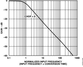
Figure 28. Typical ADC Frequency Response, Chopping Disabled
