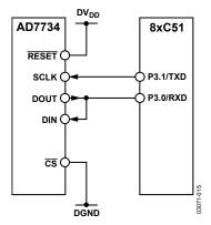
Figure 15. AD7734 to Host Device Interface, 2-Wire Configuration
