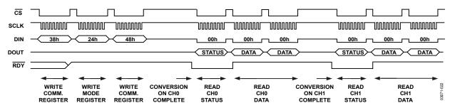
Figure 22. Continuous Conversion, CH0 and CH1, Continuous Read
