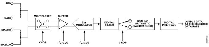
Figure 24. Channel Signal Chain Diagram with Chopping Enabled
