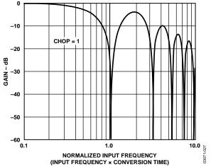
Figure 27. Typical ADC Frequency Response, Chopping Enabled
