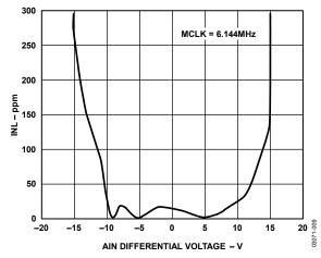
Figure 9. Typical INL vs. AIN Voltage, AIN Range =  $\pm 10 V$ , BIASO to BIAS3, BIASHI = 2.5 V, BIASLO = 0 V
