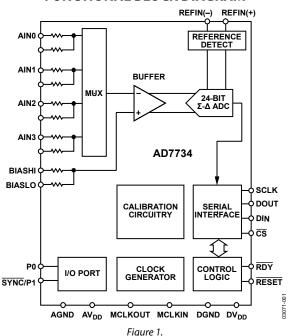
3-wire operation and is compatible with microcontrollers and digital signal processors. All interface inputs are Schmitt triggered.
