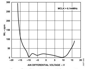
Figure 8. Typical INL vs. AIN Voltage, AIN Range  $=\pm 10 V$ , BIASO to BIAS3, BIASHI = 2.5 V, BIASLO = O V
