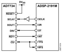
Figure 14. AD7734 to Host Device Interface, DSP
