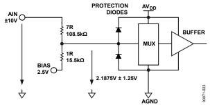
Figure 23. Simplified Analog Input Internal Structure
