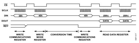
Figure 17. Serial Interface Signals—Single Conversion Command and 16-Bits Data Reading
