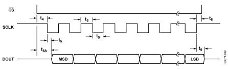
Figure 2. Read Cycle Timing Diagram
