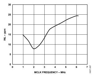
Figure 7. Typical INL vs. MCLK Frequency,  $AIN = \pm 10 \text{ V, BIASO to BIAS3, BIASHI} = 2.5 \text{ V, BIASLO} = 0 \text{ V}$
