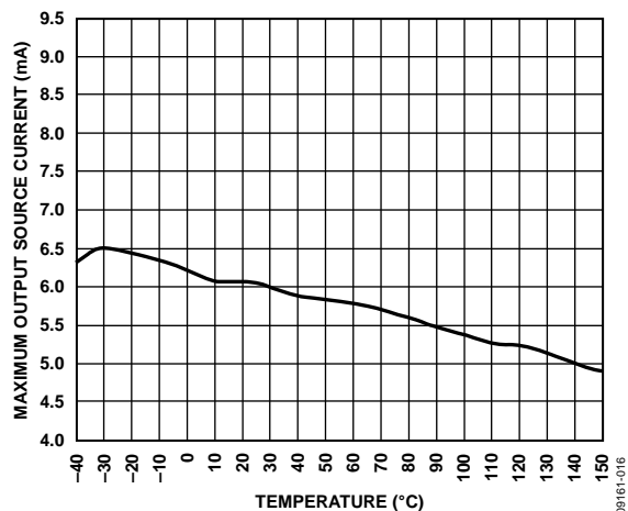
Figure 16. Maximum Output Source Current vs. Temperature
