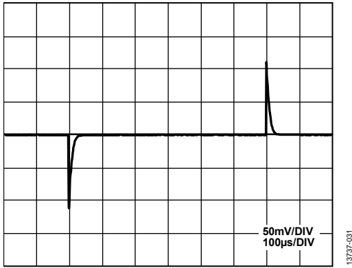
Figure 31. Load Transient Response (100 µA Load Change)
