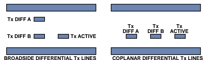
Figure 66. Broadside vs. Coplanar Differential Stripline Routing Techniques
