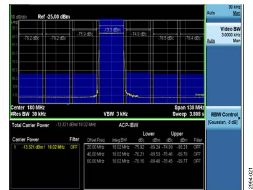
Figure 20. 1C 5 MHz Bandwidth LTE ACLR Performance, IF = 180 MHz, f_{DAC} = 1966.08 MHz
