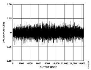
Figure 29. AD9255-105 DNL with  $f_{IN} = 12.5 \text{ MHz}$
