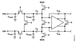
Figure 64. Switched-Capacitor Input
