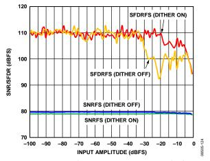
Figure 24. AD9255-105 Single-Tone SNR/SFDR vs. Input Amplitude (A<sub>IN</sub>) with  $f_{\rm IN}=30$  MHz with and without Dither Enabled
