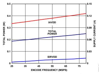
Figure 83. AD9255-80 Power and Current vs. Sample Rate
