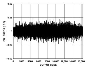
Figure 17. AD9255-80 DNL with  $f_{\text{IN}} = 12.5 \text{ MHz}$
