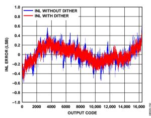
Figure 50. AD9255-125 INL with  $f_{IN} = 12.5 \text{ MHz}$
