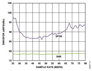
Figure 14. AD9255-80 Single-Tone SNR/SFDR vs. Sample Rate ( $f_s$ ) with  $f_{\rm IN}$  = 70.1 MHz
