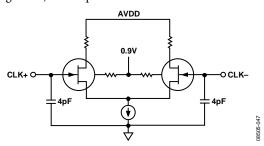
Figure 74. Equivalent Clock Input Circuit
