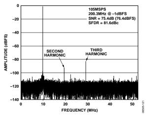
Figure 21. AD9255-105 Single-Tone FFT with  $f_{IN}$  = 200.3 MHz
