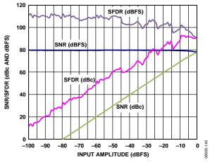
Figure 40. AD9255-125 Single-Tone SNR/SFDR vs. Input Amplitude (A<sub>IN</sub>) with  $f_{\rm IN}=98.12$  MHz
