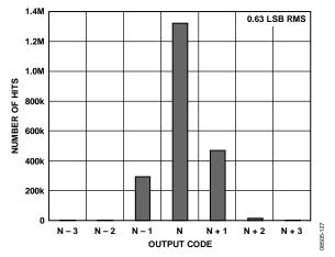
Figure 27. AD9255-105 Grounded Input Histogram
