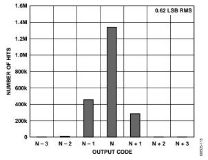
Figure 15. AD9255-80 Grounded Input Histogram
