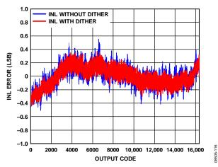
Figure 16. AD9255-80 INL with  $f_{IN} = 12.5 \text{ MHz}$
