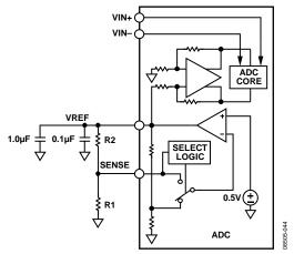
Figure 71. Programmable Reference Configuration
