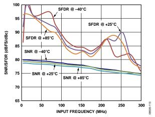
Figure 13. AD9255-80 Single-Tone SNR/SFDR vs. Input Frequency ( $f_{\mathbb{N}}$ ) and Temperature with 2 V p-p Full Scale
