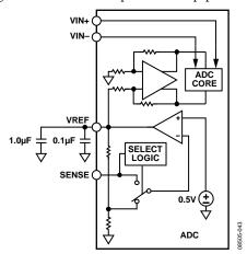
Figure 70. Internal Reference Configuration
