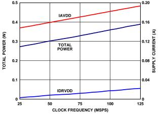
Figure 81. AD9255-125 Power and Current vs. Sample Rate
