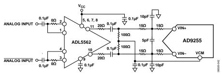
Figure 69. Differential Input Configuration Using the ADL5562
