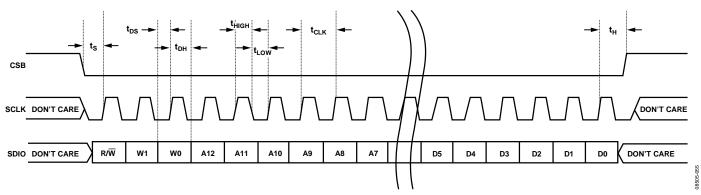
Figure 84. Serial Port Interface Timing Diagram
