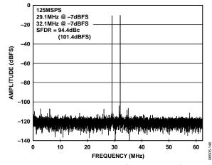
Figure 46. AD9255-125 Two-Tone FFT with  $f_{\mathbb{N}1}$  = 29.1 MHz and  $f_{\mathbb{N}2}$  = 32.1 MHz
