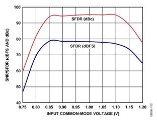
Figure 52. AD9255-125 SNR/SFDR vs. Input Common Mode (VCM) with  $f_{\rm IN}$  = 30 MHz
