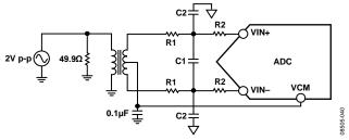
Figure 67. Differential Transformer-Coupled Configuration
