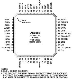
Figure 4. LFCSP Parallel CMOS Pin Configuration (Top View)
