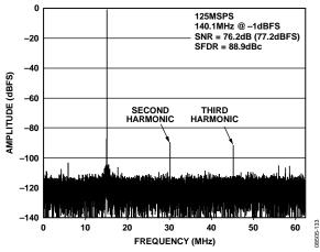
Figure 33. AD9255-125 Single-Tone FFT with  $f_{IN} = 140.1 \text{ MHz}$
