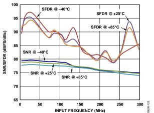
Figure 25. AD9255-105 Single-Tone SNR/SFDR vs. Input Frequency (f<sub>in</sub>) and Temperature with 2 V p-p Full Scale
