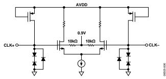
Figure 54. Equivalent Clock Input Circuit
