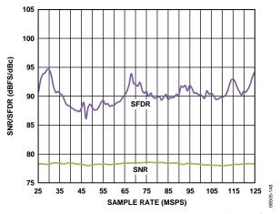
Figure 48. AD9255-125 Single-Tone SNR/SFDR vs. Sample Rate ( $f_s$ ) with  $f_{\rm IN}$  = 70.1 MHz
