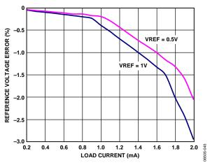
Figure 72. VREF Accuracy vs. Load
