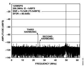
Figure 34. AD9255-125 Single-Tone FFT with  $f_{IN} = 200.3$  MHz
