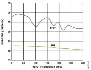
Figure 43. AD9255-125 Single-Tone SNR/SFDR vs. Input Frequency ( $f_{IN}$ ) with 1 V p-p Full Scale
