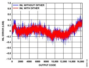
Figure 28. AD9255-105 INL with  $f_{IN} = 12.5 \text{ MHz}$
