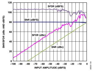
Figure 39. AD9255-125 Single-Tone SNR/SFDR vs. Input Amplitude (A<sub>IN</sub>) with  $f_{\rm IN}=2.4$  MHz
