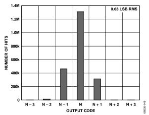
Figure 49. AD9255-125 Grounded Input Histogram
