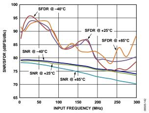
Figure 42. AD9255-125 Single-Tone SNR/SFDR vs. Input Frequency ( $f_{\text{IN}}$ ) and Temperature with 2 V p-p Full Scale
