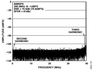
Figure 9. AD9255-80 Single-Tone FFT with  $f_{IN} = 200.3$  MHz
