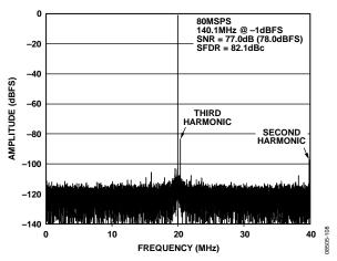
Figure 8. AD9255-80 Single-Tone FFT with  $f_{IN} = 140.1 \text{ MHz}$
