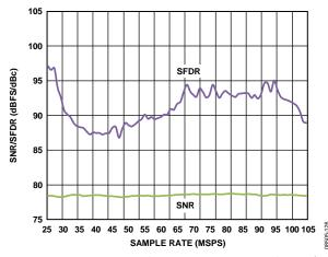
Figure 26. AD9255-105 Single-Tone SNR/SFDR vs. Sample Rate ( $f_s$ ) with  $f_{\rm IN}$  = 70.1 MHz
