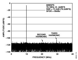
Figure 10. AD9255-80 Single-Tone FFT with  $f_{\rm IN}$  = 70.1 MHz at -6 dBFS with Dither Enabled
