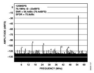
Figure 37. AD9255-125 Single-Tone FFT with  $f_{\rm IN}$  = 70.1 MHz at -23 dBFS with Dither Disabled, 1M Sample
