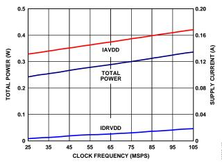
Figure 82. AD9255-105 Power and Current vs. Sample Rate
