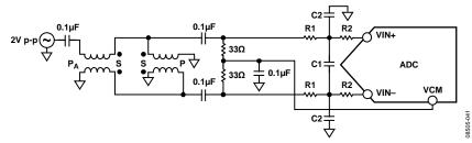
Figure 68. Differential Double Balun Input Configuration
