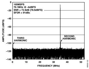
Figure 22. AD9255-105 Single-Tone FFT with  $f_{\rm IN}$  = 70.1 MHz at -6 dBFS with Dither Enabled
