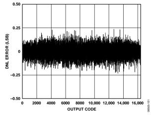
Figure 51. AD9255-125 DNL with  $f_{IN} = 12.5 \text{ MHz}$
