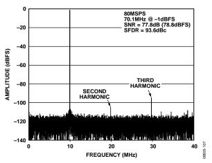
Figure 7. AD9255-80 Single-Tone FFT with  $f_{IN} = 70.1$  MHz
