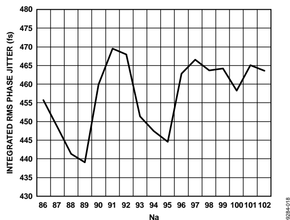
Figure 18. Typical Integrated Random Phase Jitter in fs rms for PLL1 and OUT0P LVPECL as Feedback Divider Value Na Swept ( f_{XTAL} = 25 MHz, V0 = 5 , D0 = 5 )
