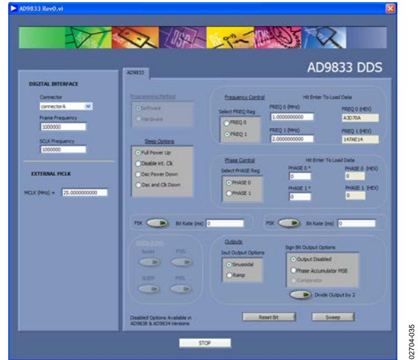
Figure 33. AD9833 Evaluation Software Interface
