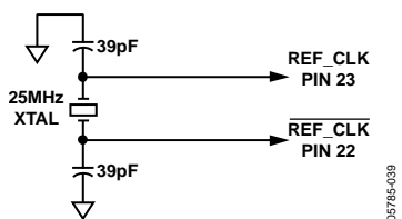
Figure 40. Crystal Configuration for Reference Clock Source
