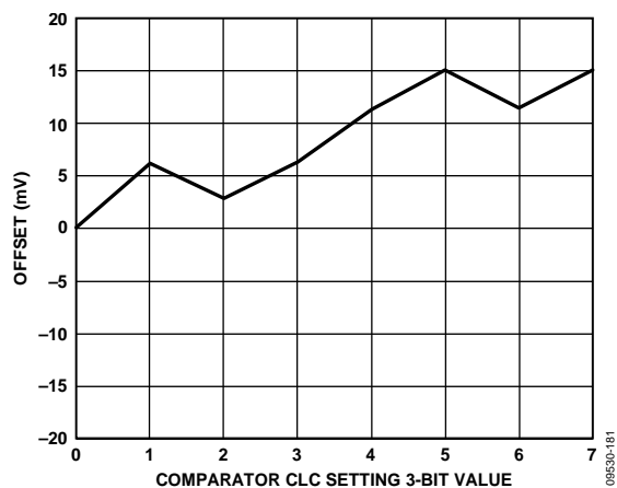
Figure 88. Normal Window Comparator Offset Error vs. CLC Setting
