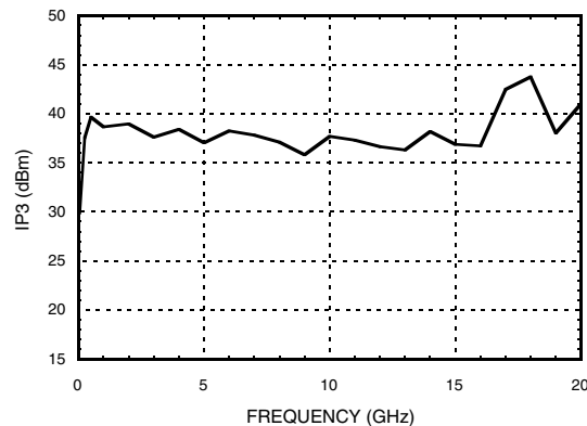
Input Third Order Intercept Point @ 0 dBm Tone Power
