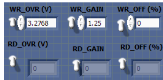
Figure 16. Overrange, Gain, Offset register Write and Read functions.
