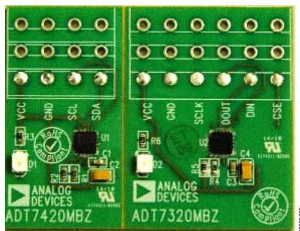
Figure 2. ADT7x20 Evaluation Board—External Board
