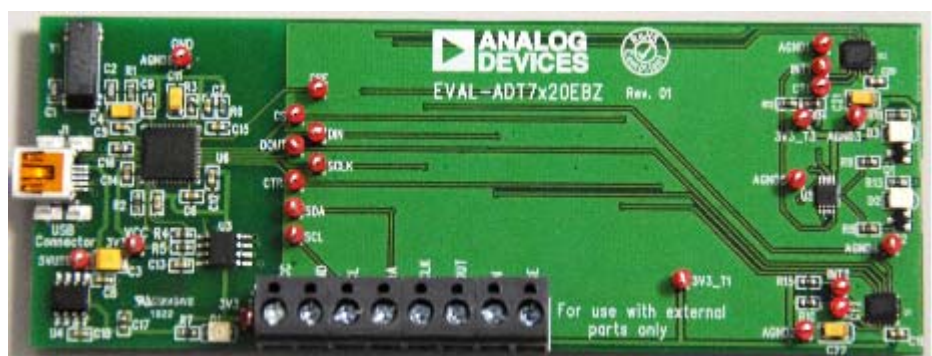
Figure 1. ADT7x20 Evaluation Board—Main Board
