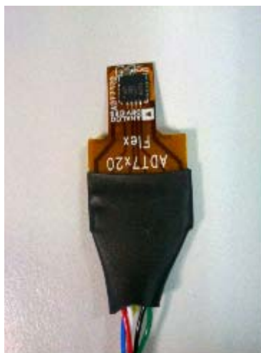
Figure 3. ADT7320FBZ Evaluation Board—External Board
