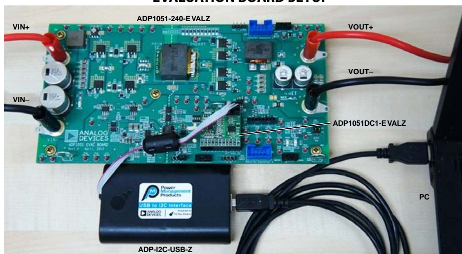
Figure 1. ADP1051 Evaluation Board Setup
