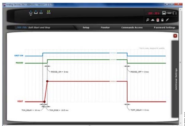
Figure 13. Soft Start and Stop Settings Window
