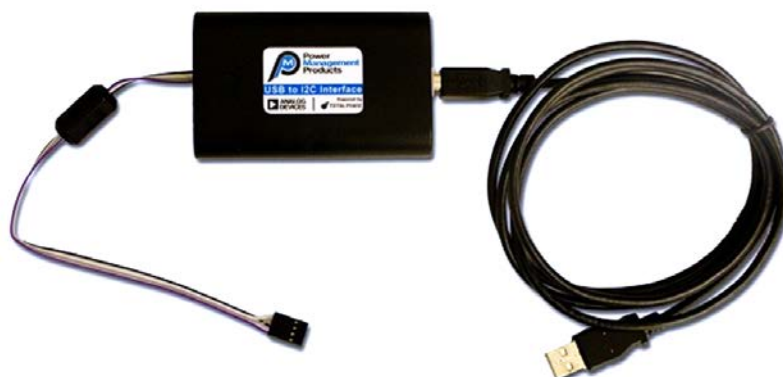
Figure 5. ADP-I2C-USB-Z USB-to-I 2 C Interface Connector
