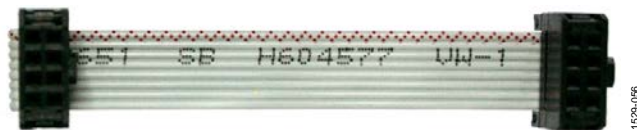
Figure 55. Parallel Cable to Connect Two Evaluation Boards
