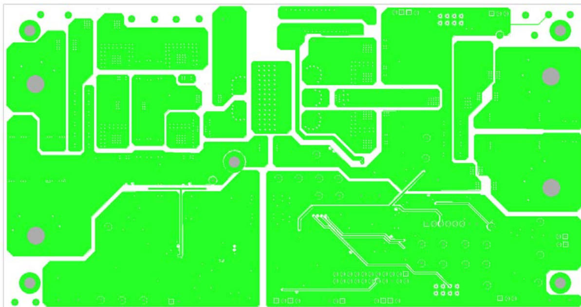
Figure 67. PCB Layout, Layer 2
