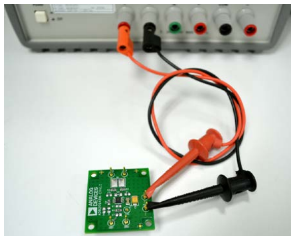
Figure 3. Basic Power Connections of the AD8209A Evaluation Board
