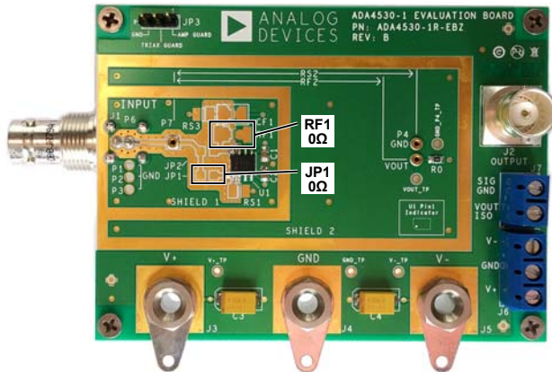
Figure 5. Buffer with Triax Guard Externally Driven
