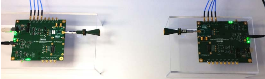
Figure 10. Typical HMC6300 and HMC6301 60 GHz Radio Link
