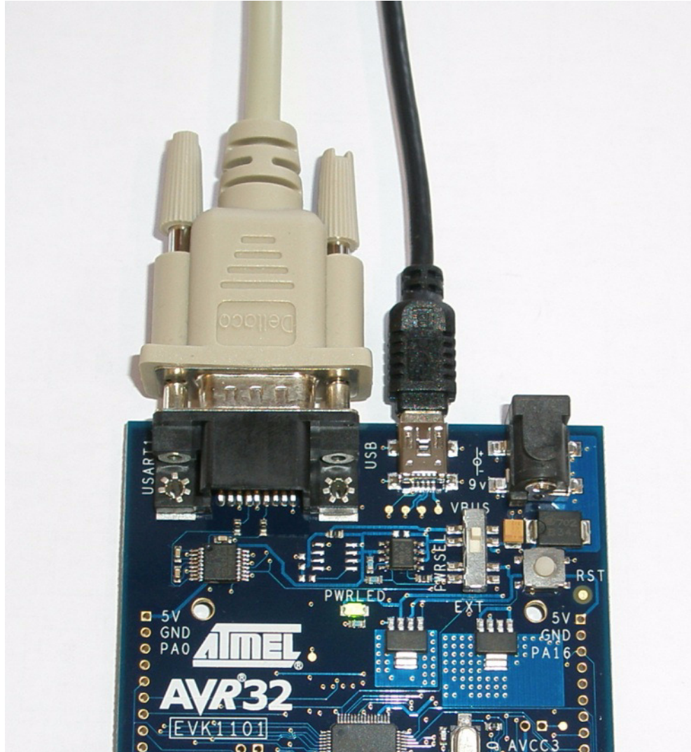
Figure 4-2. Powering the EVK1101 using the USB cable
