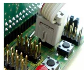
3. Plug an USB level converter into a free USB port on your PC. Interconnect this level converter and one of both REB-CBB assemblies via the 6pin ribbon cable such that it fits the notch on the level converter and the colored stripe of the ribbon cable connects to pin 1 of the CBB header, USARTD0.
