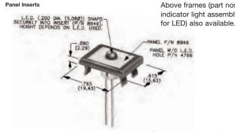
Above frames (part nos. 432XXXXX) are also available with insert which accepts LED for indicator light assembly. Order insert separately from frame. Blank insert panel (without hole for LED) also available. LED not included.
