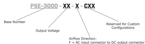
B = DC output connector to AC input connector
