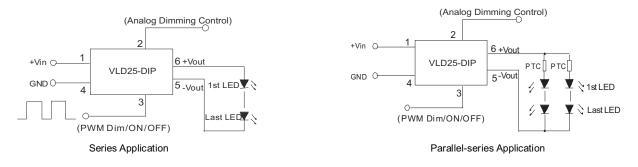
To protect the LED(s), you could connect a PTC to input of all channels as shown in application circuit. Note: Negative output terminal should not conneted to GND. Module may be damaged.
