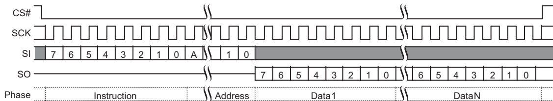
Figure 9.28 Read Command Sequence (3-Byte Address, 03h or 13h)
