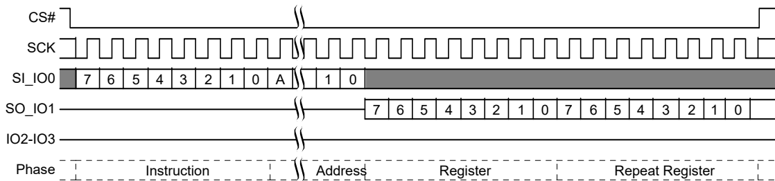
Figure 110. PPB Read Command Sequence
