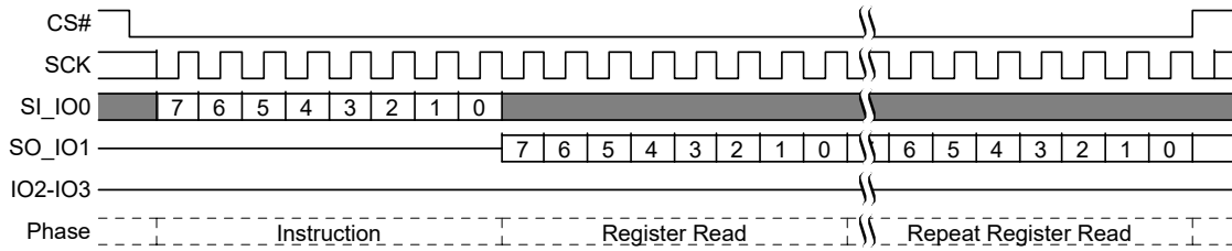
Figure 56. Read Configuration Register (RDCR) Command Sequence
