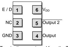
Terminations as viewed from the Top NOTE: XPRESSO LVDS XOs are designed to fit on Industry Standard, 6 pad layouts
