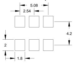
Note: XPRESSO LVDS XOs are designed to fit on Industry standard, 6 pad, layouts.
