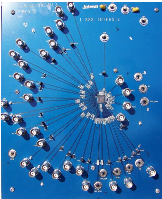
FIGURE 4. ISL55100A/BEVAL3/3Z EVALUATION BOARD
