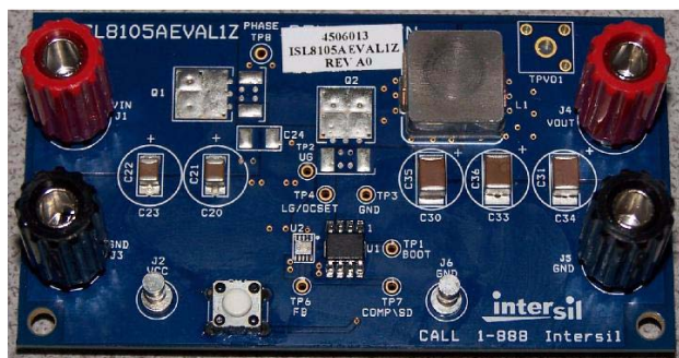
FIGURE 1. ISL8105AEVAL1Z EVALUATION BOARD
