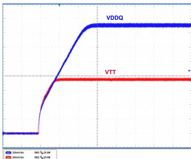
FIGURE 18. VDDQ AND VTT START-UP TRACKING (DDR3)
