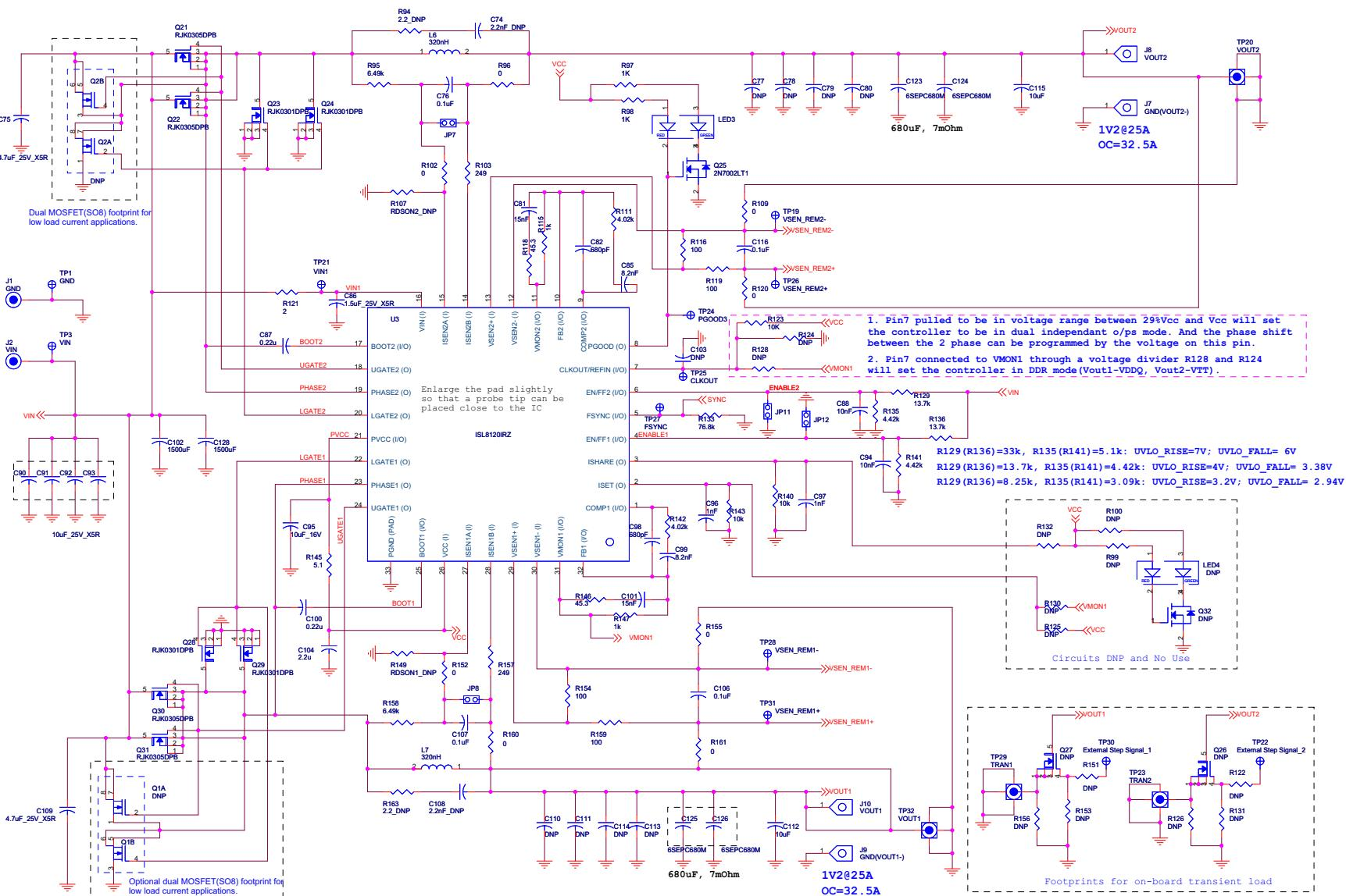
FIGURE 3. ISL8120EVAL3Z SCHEMATIC
