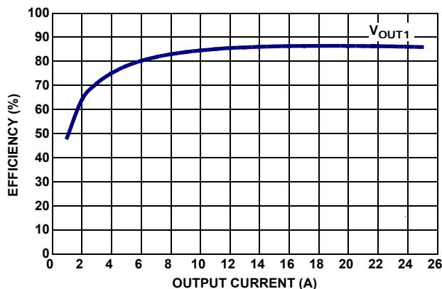
FIGURE 11. CHANNEL 1 EFFICIENCY (12V  $V_{IN}$  AND 1.2V  $V_{OUT}$ )
