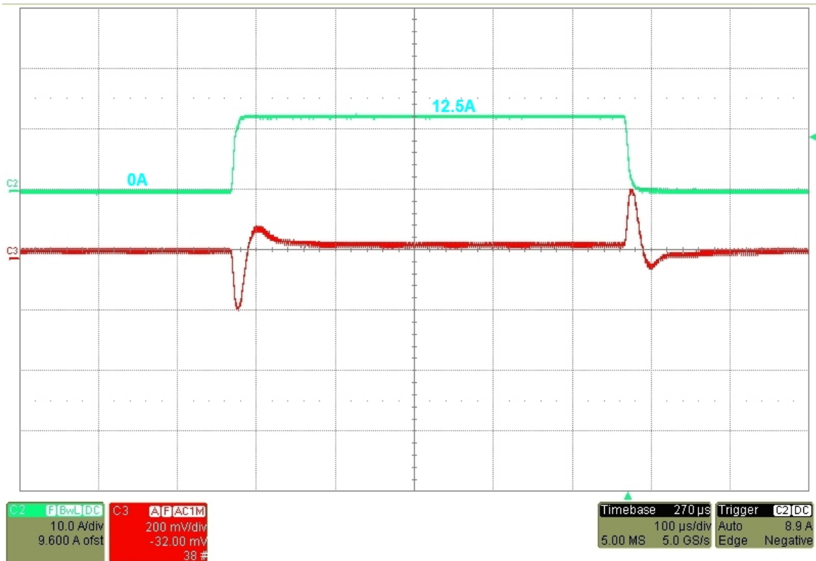
FIGURE 23. STEP LOAD: 0A TO 12.5A (12.5A DELTA)
