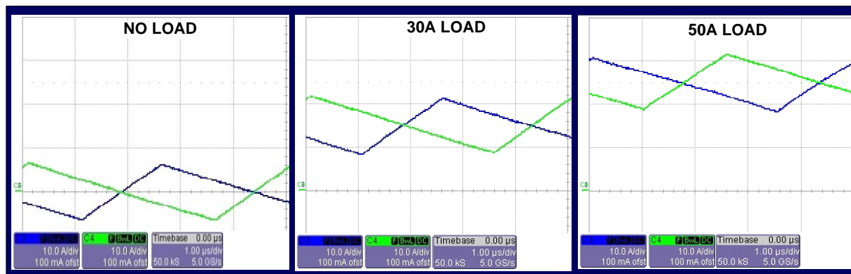
FIGURE 14. INDUCTOR CURRENT WAVEFORMS
