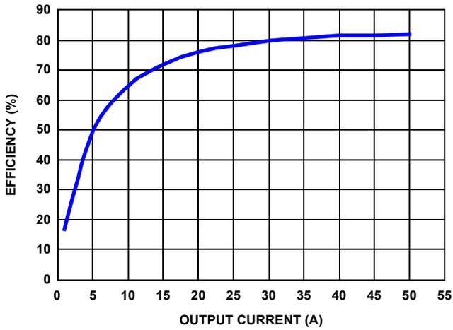
FIGURE 13. EFFICIENCY (12V  $V_{IN}$  AND 1.2V  $V_{OUT}$ )
