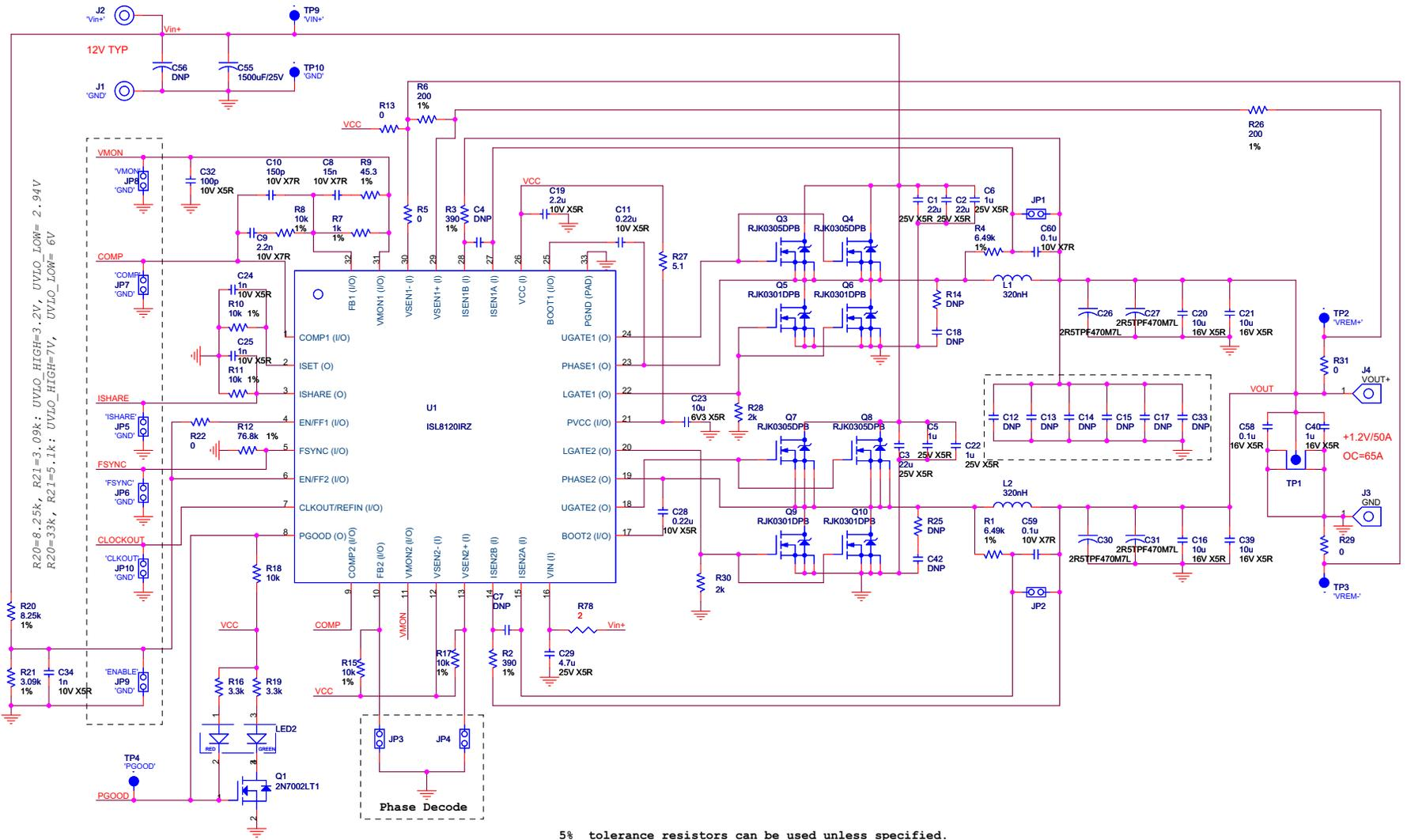
FIGURE 3. ISL8120EVAL4Z SCHEMATIC
