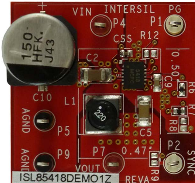
FIGURE 6. ISL85418DEMO1Z DEMONSTRATION BOARD (TOP)
