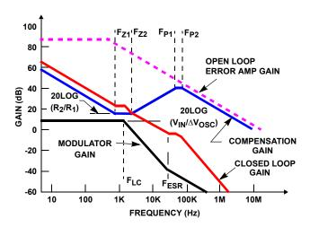
FIGURE 4. ASYMPTOTIC BODE PLOT OF CONVERTER GAIN
