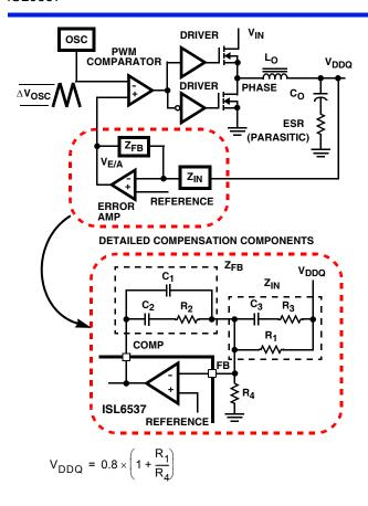
FIGURE 3. VOLTAGE-MODE BUCK CONVERTER
