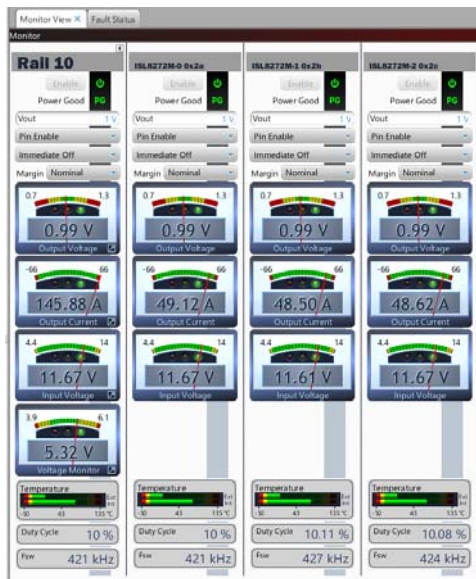
FIGURE 21. STATIC CURRENT SHARING MONITORED FROM THE POWERNAVIGATOR SOFTWARE, V_{IN} = 12V , V_{OUT} = 1V , I_{OUT} = 150A , f_{SW} = 421kHz
