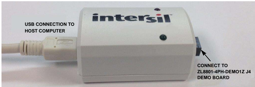
FIGURE 13. USB TO PMBus DONGLE
