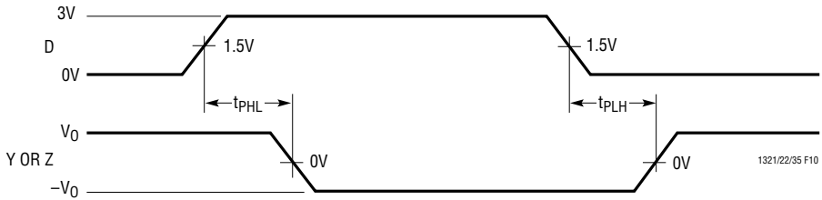
Figure 10. EIA/TIA-562 Driver Propagation Delays
