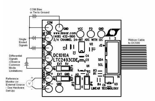
Figure 1. Proper Measurement Equipment Setup
