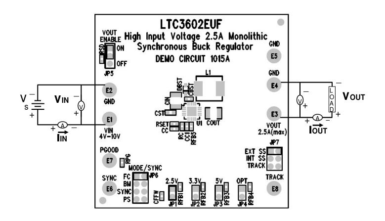
Figure 1. Proper Equipment Measurement Set-Up
