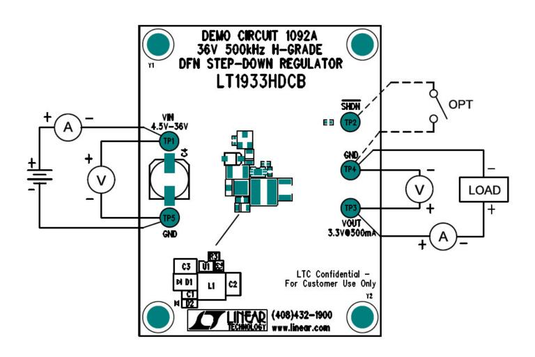
Figure 1. Proper Measurement Equipment Setup
