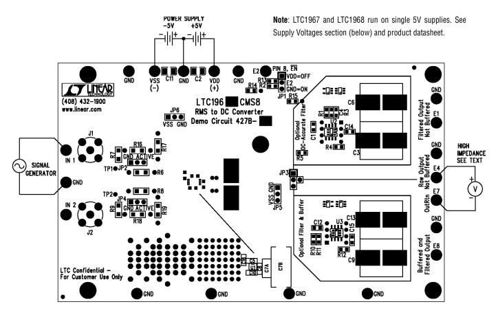
Figure 1. Proper Measurement Equipment Setup
