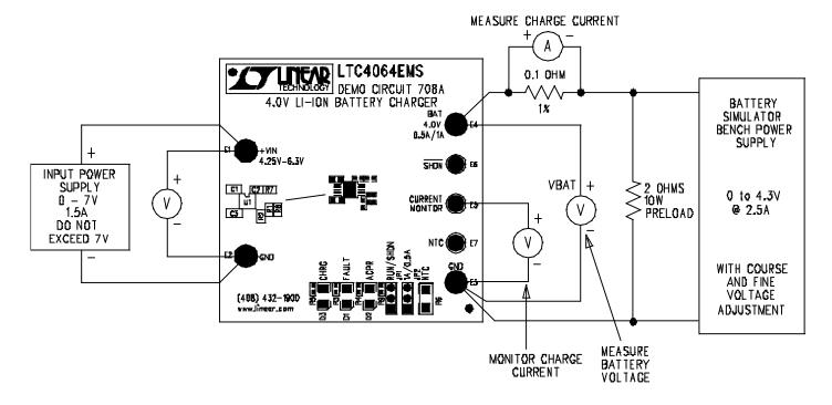
Figure 1. Proper Measurement Equipment Setup
