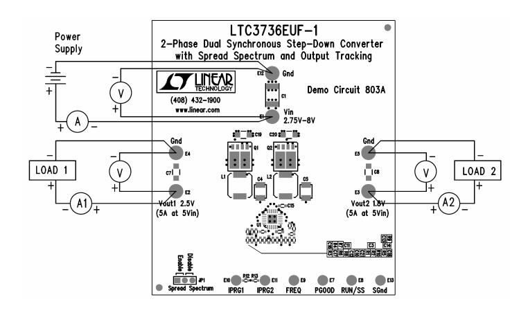
Figure 1. Proper Measurement Equipment Setup
