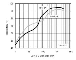
Figure 2. Efficiency vs load current (550kHz)
