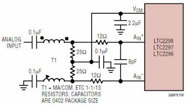
Figure 3. Analog Front End Circuit For 70MHz  $< A_{IN} < 170MHz$  (1 of 2)
