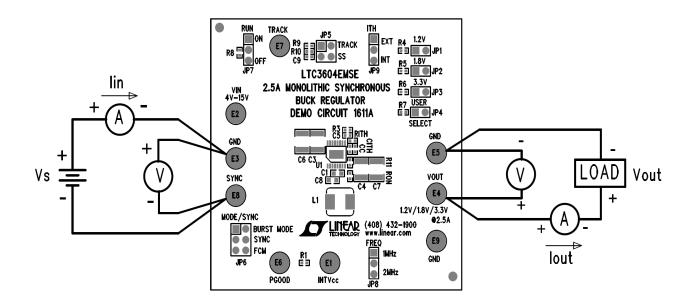
Figure 1. Proper Equipment Measurement Set-Up
