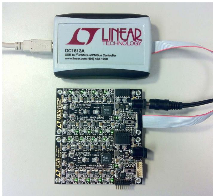
Figure 12. Array of Multiple DC2028A Demo Boards
