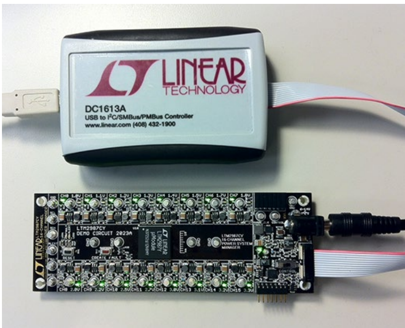
Figure 2. Connecting DC2023A board and the DC1613 I 2 C/SMBus/PMBus Controller
