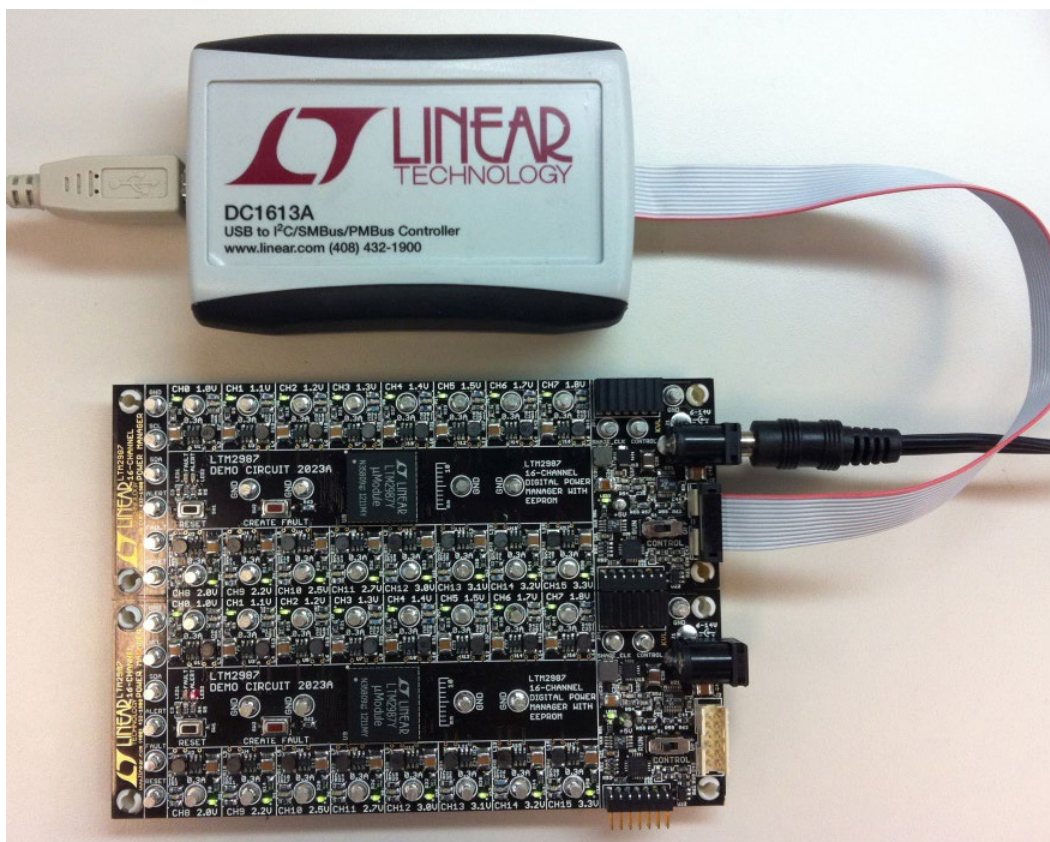
Figure 12. Array of Multiple DC2023A Demo Boards
