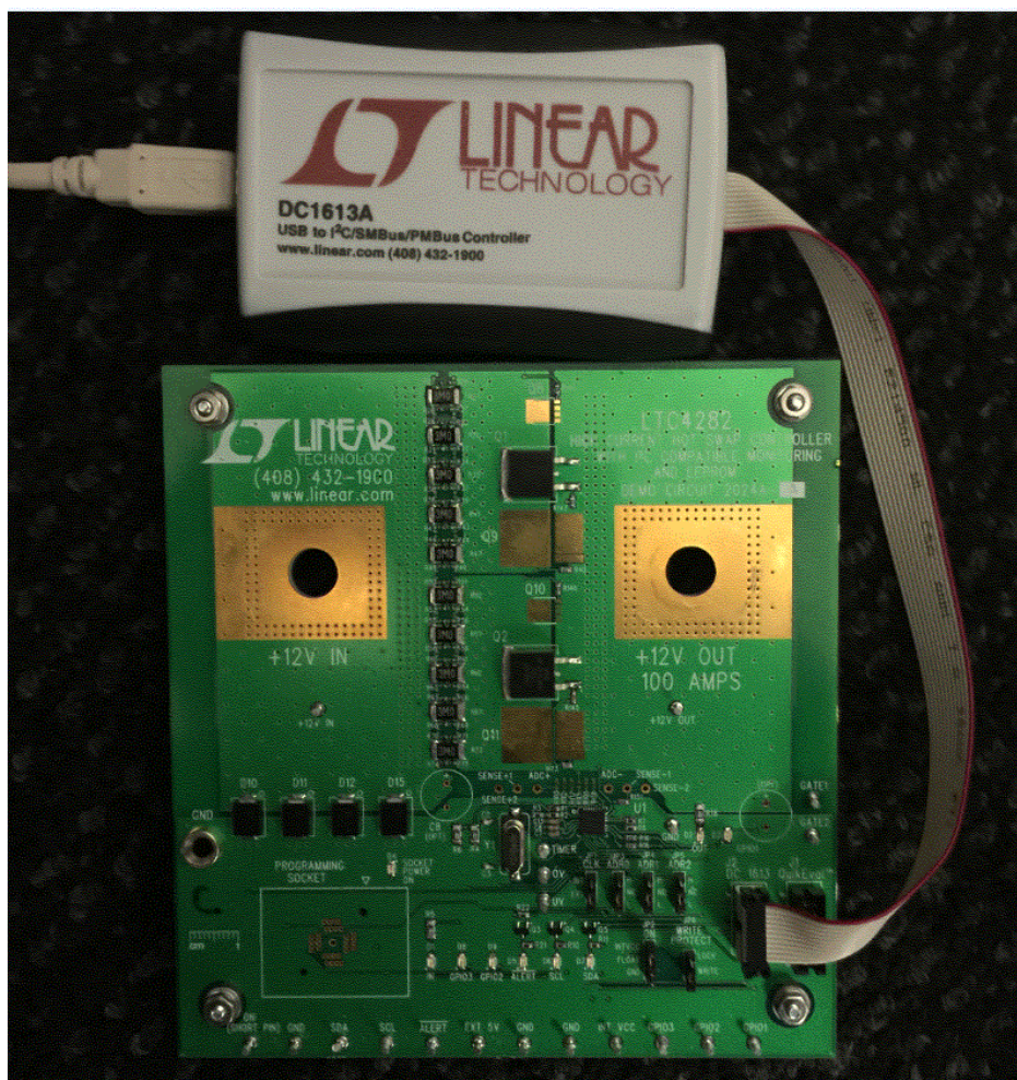
Figure 2. DC2024A-A Demo Board Connected to DC1613 I 2 C-to-USB Converter
