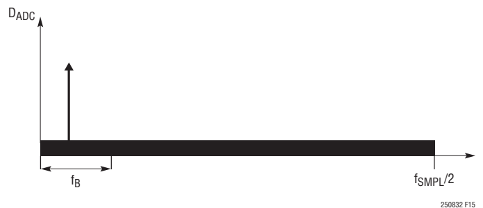
Figure 15. Frequency Spectrum of SAR ADC Core Output
