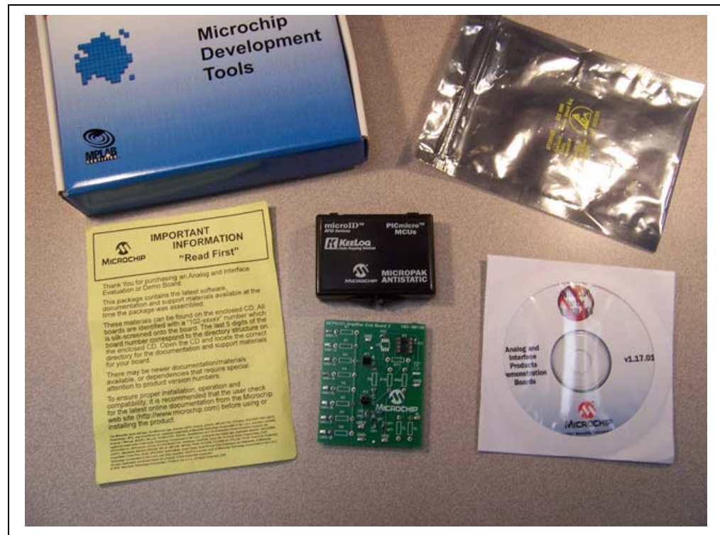
FIGURE 1-1: MCP6XXX Amplifier Evaluation Board 2 Kit.
