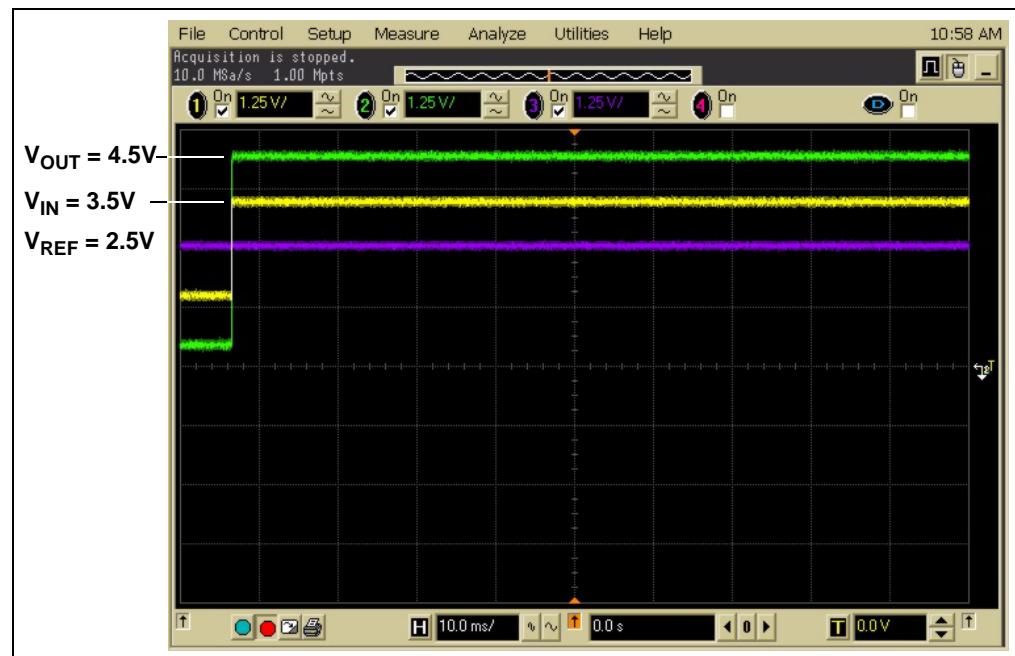
FIGURE 2-14: Measured Step Response.
