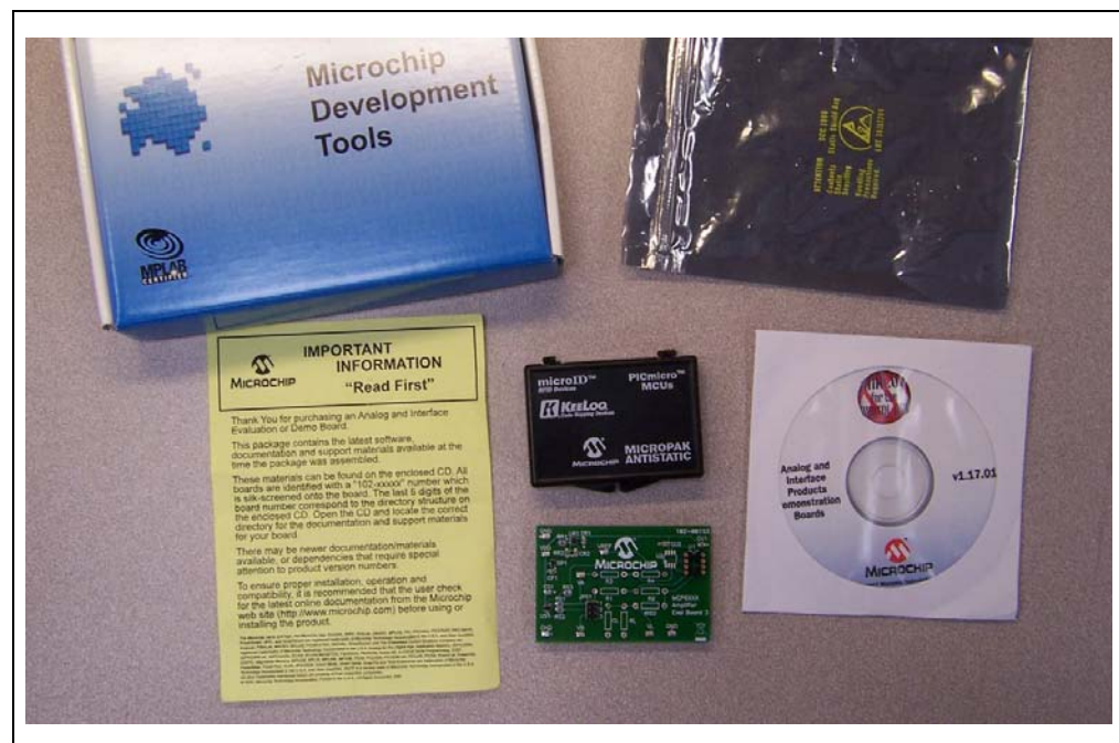
FIGURE 1-1: MCP6XXX Amplifier Evaluation Board 3 Kit.
