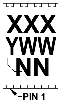
8-Lead UDFN (2x3x0.5 mm)
